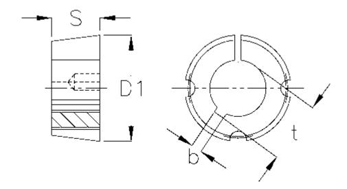
b = 6 Bore = 20 = 1215 Bush type = 47,5 D1 = 38,1S Screw size  $= 3/8 \times 5/8$ " = 22.8
